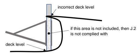
The design described in the AYRA RFI is not the situation described in the Q&A relating to Walicki type masts as, in this case, the mast is a continuous element without a break.
